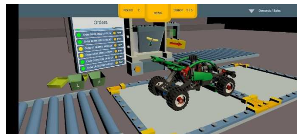
Fig1. Station in the tablet application of the game LEAN40SG, where a student assembles his component from Lego pieces according to a manual, monitors the stock level, and orders transport to the next station, where another student is already playing. The goal is to assemble as many cars as possible in the given time in 4 rounds where elements of lean methods are introduced, and virtual helpers are added in the form of industry 4.0 elements such as collaborative robots or 3d printers, predictive maintenance, and others.
